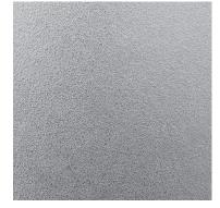
a heat tint scale may be avoided in lighter gauges. When scale does form, care must be taken to remove this scale through mechanical or chemical means. Because Starlight is non-directional, there is no need to orient panels in relation to the rolling direction. Still, to avoid the possible result of slight directional differences, we suggest panels be fabricated to maintain the alignment of the original sheet. After soldering, flux residue must be thoroughly removed.
